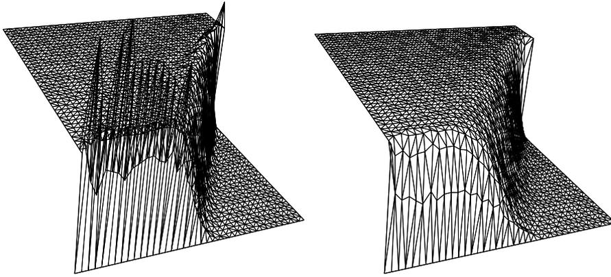
FIGURE 5. Outflow boundary layer testcase using ES, left without shock capturing, right with shock capturing
