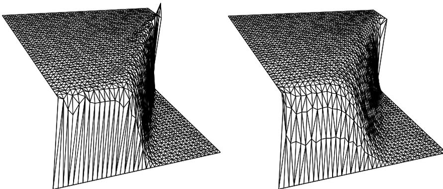
FIGURE 4. Outflow boundary layer testcase using SD, left without shock capturing, right with shock capturing
