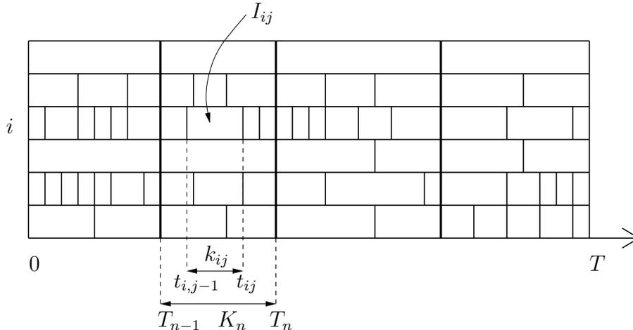
FIGURE 1. Individual partitions of the interval  $(0, T]$  for different components. Elements between common synchronised time levels are organised in time slabs. In this example, we have  $N = 6$  and  $M = 4$ .
