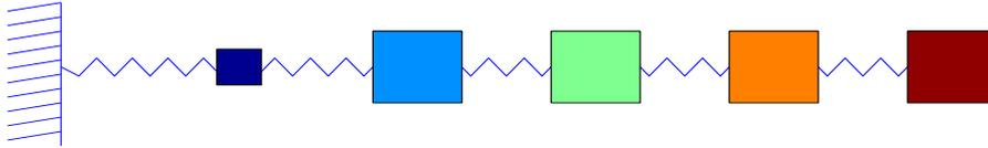
FIGURE 3. A mechanical system consisting of  $N = 5$  masses attached together with springs.
