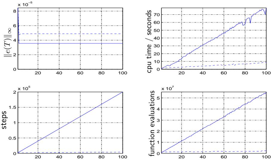
FIGURE 4. Error, cpu time, total number of steps, and number of function evaluations as function of the number of masses, for the multi-adaptive cG(1) method (dashed) and the standard cG(1) method (solid).
