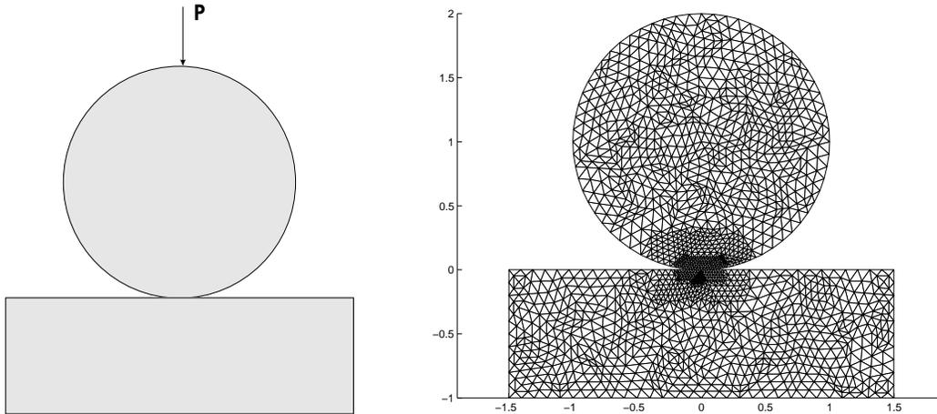
FIGURE 1. Hertz contact - Cylinder and a plane.
