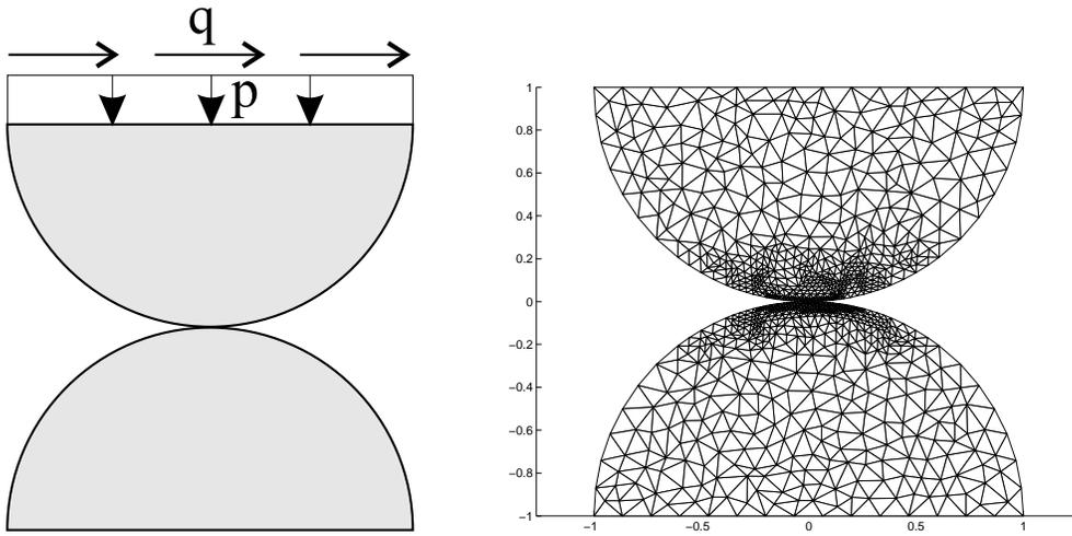
FIGURE 3. Contact between two cylinders
