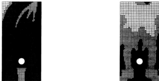
Figure 1.2: Meshes with 5,000 cells obtained by the vorticity indicator (left) and the new DWR indicator (right).
