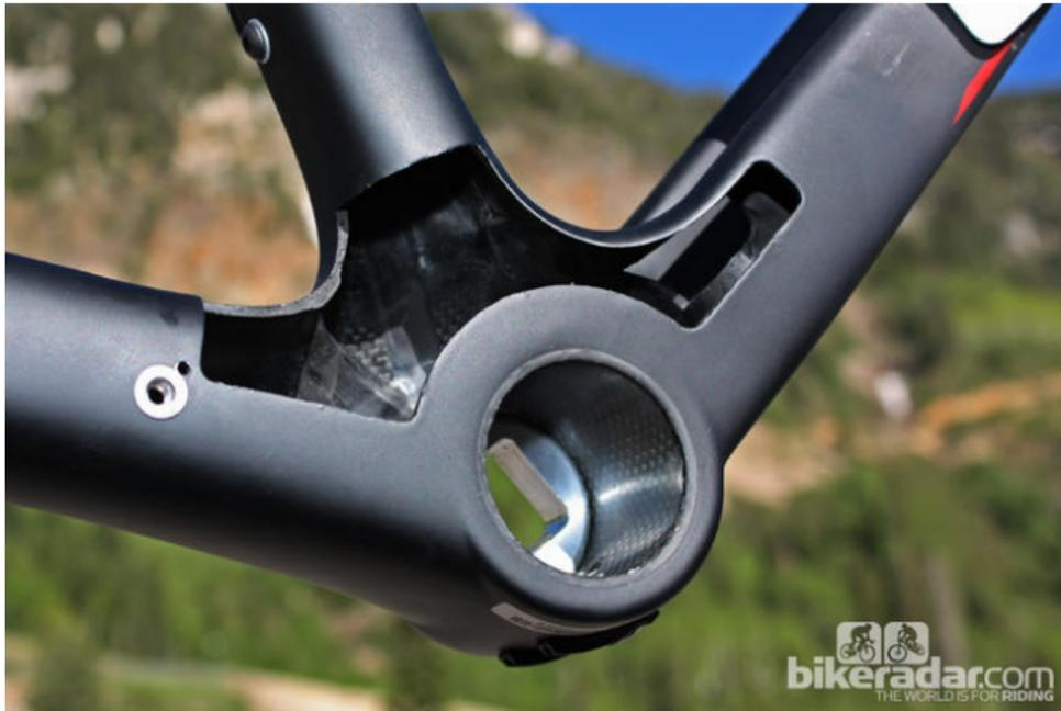
Figure : Specialized OSBB bottom bracket. Source: bikeradar.com
